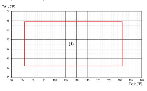
To\_h (°F) = Hot side exchanger outlet water temperature To\_c (°F) = Cold side exchanger outlet water temperature
