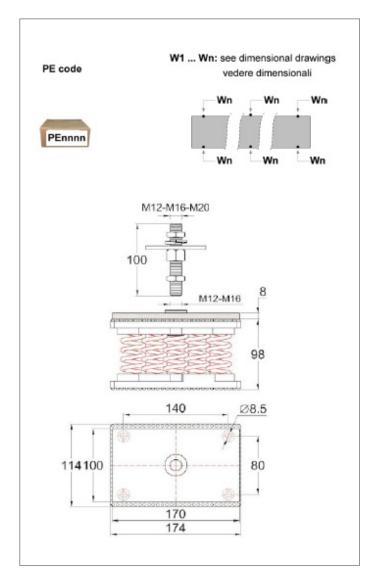
► The detail of the composition of the anti-vibration kit selected for the ordered unit (called PE.....) with details relating to each individual support point (W1, W2, etc.), is available inside the anti-vibration box shipped together with the unit.
