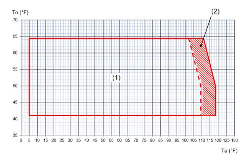
Ta (°F) = External exchanger inlet air temperature (D.B.) To (°F) = Internal exchanger outlet water temperature
